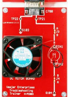
**DC Motor Circuit Kit, H-113 contains:** (1 ea.) DC Motor Circuit Board-Part Number **H-PCB03** shown at left connected to the Power Board. Resistor Bag, Part Number H-RB03 for voltage drop problems is included along with one copy of Technician Workbook, **H-WB113** and Instructor Guide, **H-IG113**.
