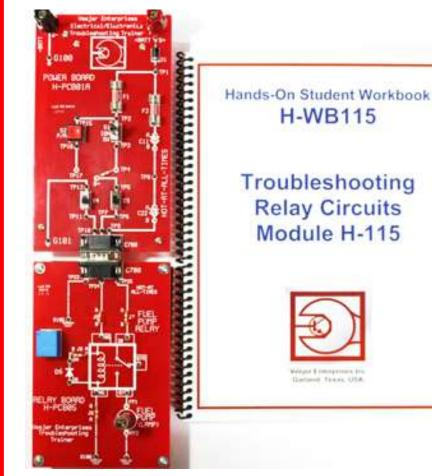
Relay Circuit Trainer H-PCB05 connects to the Power Board to complete the relay circuit for live relay circuit testing and troubleshooting.
