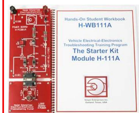
Workbook H-WB111A guides students through exercises with hands-on practice covering circuit operation and circuit testing methods with a DMM. Exercises include measuring circuit voltage, voltage drops and tracing voltage through the circuit.
