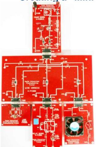
Wire Harness Electrical Trainer H-PCB06 creates a mini-electrical system (The M.E.S.) to demonstrate how the wire harness connects all circuits together into an electrical system. Illustrates with hands-on how electrical problems affect individual circuits.
