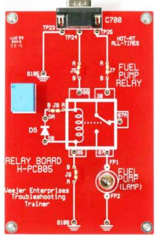
Relay Circuit Electrical Trainer H-PCB05 demonstrates how relay circuits work, how they fail and how to troubleshoot relay circuits.
